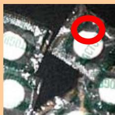
Broken tablets were blister-packed with intact tablets. In the case of a well controlled production line, the broken tablets should have been eliminated. This is an example of sub-standard quality.
